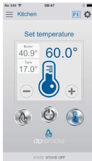
In this page, available by pressing the button in the right, you can see in real time the ambient/boiler temperature (in the top-left square, based on if the board is air (ambient) or hydro
