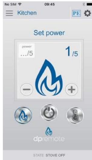
In this page, available by pressing the button in the left, you can see in real time the current working power (in the top-left square), and set the desired power by pressing the + and – buttons.
