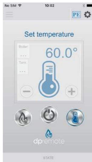
As shown, the application has established a connection with the WiFi module, but can't communicate with the electronic board because they use different protocols, so it's impossible to control the stove/boiler. In this case is sufficient to go to the protocol panel and disable it.
